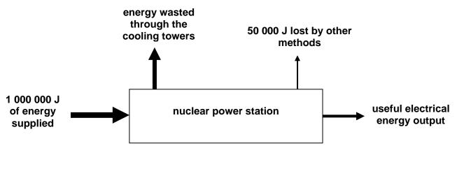
The power station has an electrical efficiency of 0.35 (35%).
